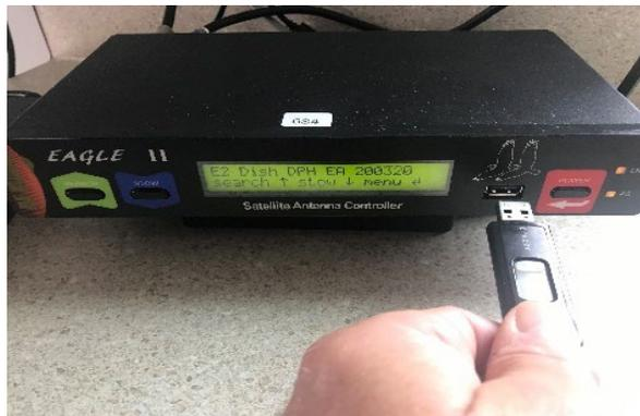
15. **Press** the POWER button to get into the MENU OPTIONS. Push the SEARCH or STOW button to get to the MENU ITEM that says TEST DISH. At this MENU ITEM hit the POWER button again and the controller will execute the TEST DISH function and connect the new software with the ANTENNA UNIT.
