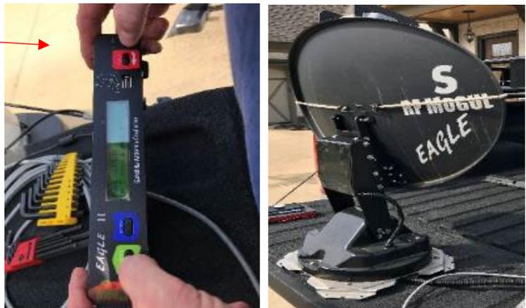
2. **Unplug** your controller before working on the antenna. Pull the 12V barrel jack out of the backside of the controller. The PS LED on the front should turn OFF.
