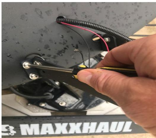
7. **Attach** the new LNB Arm loosely to the Reflector using 4 of the ¼ x 20 x ¼ inch screws provided. The LNB Arm should be able to pivot upwards into the Reflector after it is installed. Tighten all four (4) screws down tight at this point.
