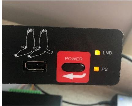
14. (If you are receiving a new controller, the software is already preloaded, so you will not receive a USB jump drive for it. Go to the next step) Power the RF Mogul antenna controller back **ON** and insert the USB JUMP Drive that has the RF Mogul antenna controller software loaded on it. The LCD display should change and show that the software is downloading. When the software download is complete, remove the USB JUMP drive.
