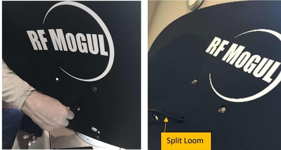
8. **Attach** the Reflector loosely to the Brackets on the Mount in the top 2 holes using 2 of the 1/4"-20 x 3/4" Philips SS screws that are provided. Align the remaining 4 holes then tighten the top 2.
