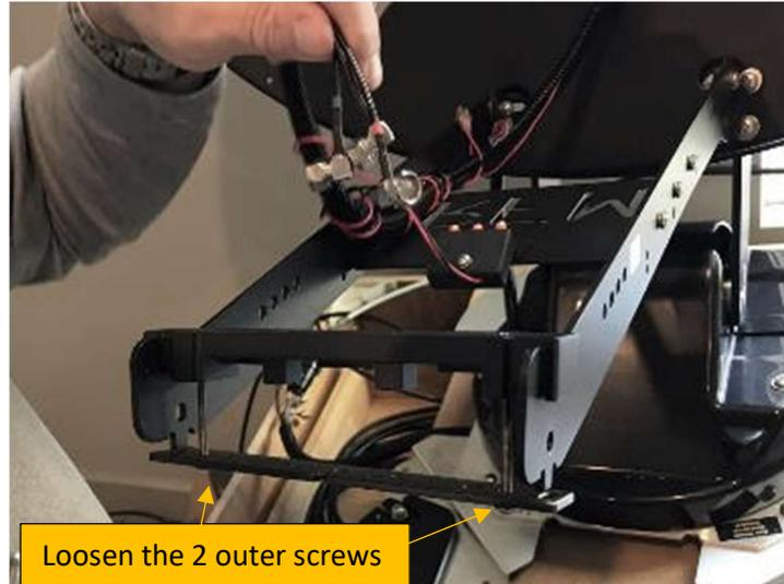
16. **Route** the LNB cable “through” the LNB brackets and attach to the LNB securely, but do not use excessive force to tighten these connectors or damage to the coax cable may occur. **Slide** the LNB into the LNB Brackets and insert the two (2) screws back into the LNB.
