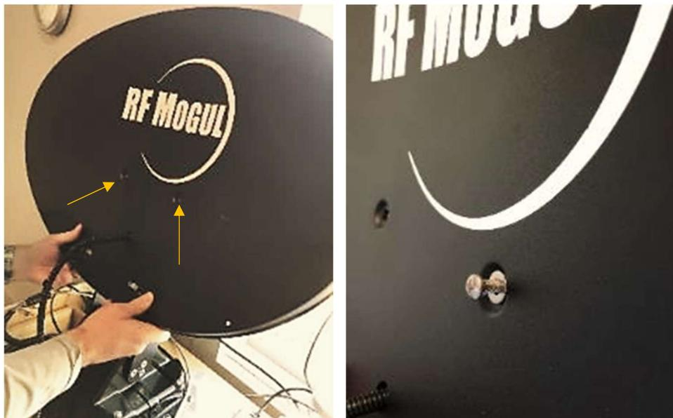
9. **Attach** the LNB Arm (choose your direction on Page 13 based on your provider) loosely to the Reflector using 4 of the 1/4" - 20 x 3/4" screws provided. The LNB Arm should be able to be pivoted upwards into the Reflector after it is attached. Tighten all 6 screws using a #3 Philips screwdriver.
