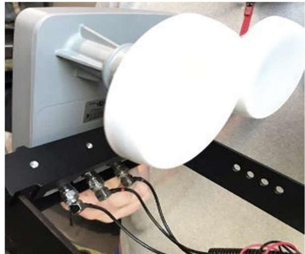
17. **Attach** the two (2) LNB Arm Stow Brackets on the inside of the LNB arm assembly (see diagram below to determine **direction** arm brackets and LNB should be placed) using the screws provided and then **secure** both the *two inner* and *outer screws* that hold the LNB into place.
