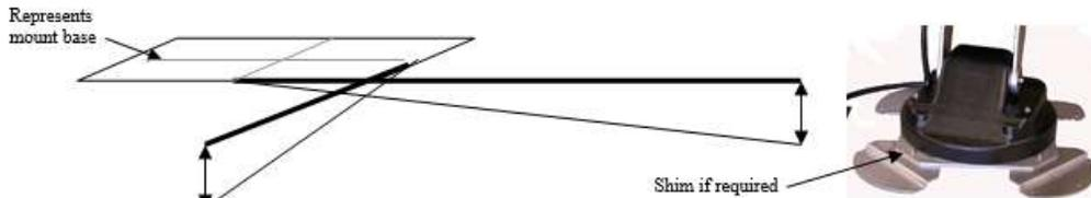
**How to measure**.... using a level, lay it onto the base of the mount. Bring the bubble of the level to center and at 12" from the center of the mount measure the distance from the bottom of the level to the roof top. If the distance 12" out from center of the mount is *less than 5/8"* or less than *1 1/4" at 24" out*, then you are within tolerance.
