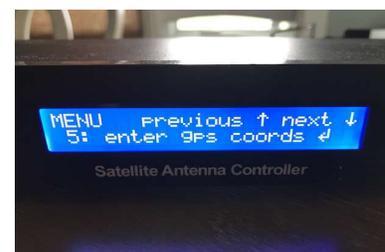
4. The LAT setting will come up first. Use the SEARCH button to move the number higher and the STOW button to move the number lower. Move the LAT to the number you have determined for your location, then press the POWER button.
