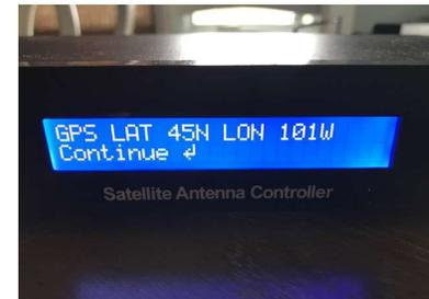
7. At this time, you can either hold the POWER button down to turn off the controller or navigate to the EXIT menu option using the SEARCH or STOW command button.
