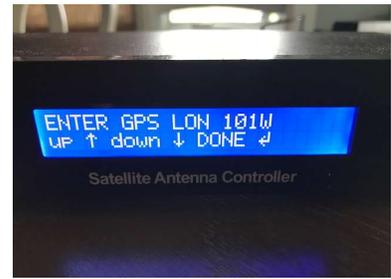
6. After LAT and LON have been entered, exit the GPS setting menu by pressing the POWER button again.
