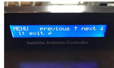
3. Once you are in the MENU use the SEARCH button to move down to option 5: Enter GPS Coords. Push the POWER button again and this will open the GPS Coordinates Menu.
